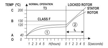
On the chart above, the interval OA represents the maximum ambient temperature, and OB is the temperature reached under normal operating duty. In case there is any failure with further rotor locking, the condition is represented on the interval 2 of the chart. The motor temperature increases fastly up to interval OC which must be shorter than motor classification temperature T. So, care must be taken to ensure motor is switched-off within time tE.
